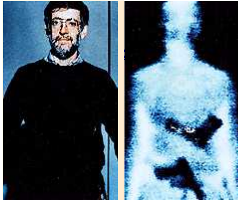
Millimeter-wave camera picks up both metallic and plastic concealed handguns.
